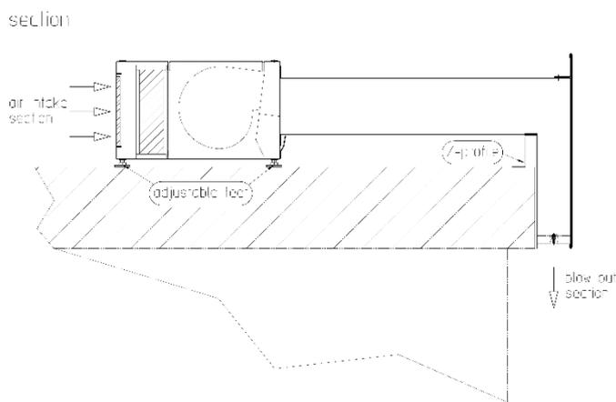
The air curtain is fitted on the crown of the revolving door and is horizontally adjusted using the adjust-able feet.
