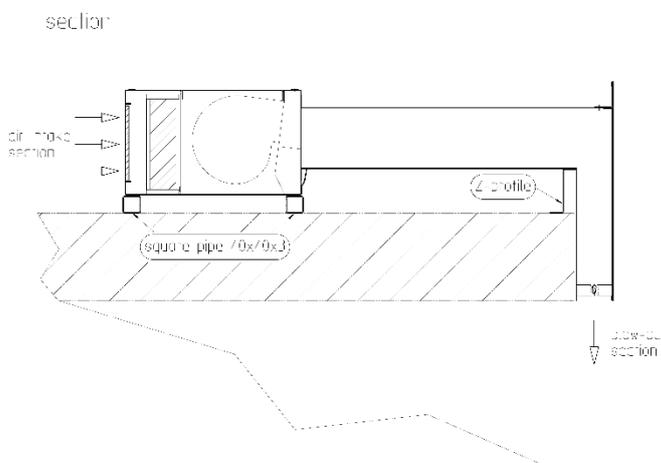
If the crown of the revolving door cannot support the weight of the air curtain, mounting with square pipes is a useful alternative.
