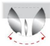
The air discharge angle of the nozzle can be finely adjusted by hand or by means of grids. To obtain maximum screening the nozzle must be directed according to requirements.
