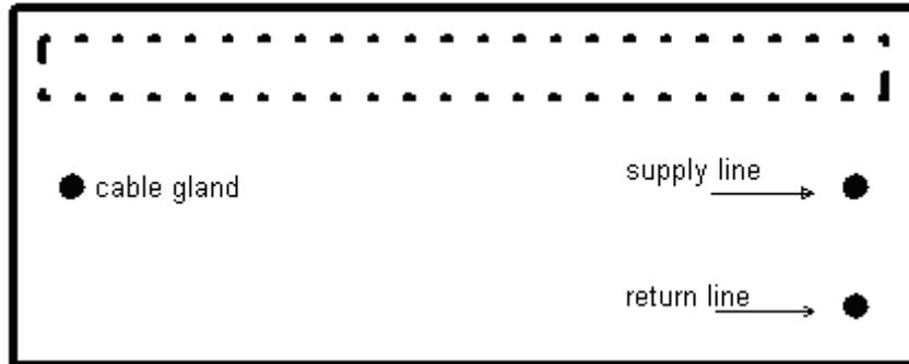
The heater battery connections for warm water operation are located at the top of the unit. Flow/reverse flow runs are marked. Cable glands for connecting the motors to the power supply are also located on the top of the system. For systems with electrical heating elements, the cable gland is located on the top of the system. Other connection options are available on request.
